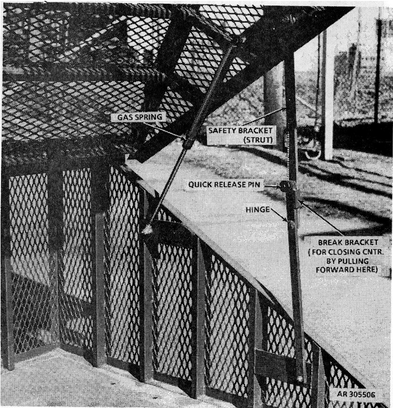
Figure 1-5. Details of Support Bracket and Gas Spring
